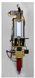
The LITEStream shot meter package is ideal for single-component applications where the overall volume of each dispense is less than 70 cc's. With this configuration, material is pre-filled and the material chamber is pressurized with a metering rod. Dispensing is constantly controlled and monitored by a pressure transducer that verifies material flow and continuously makes adjustments to maintain a **consistent** and **uninterrupted** flow rate during application.
